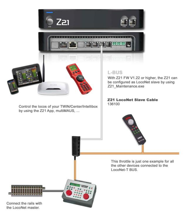
This digital command station is the LocoNet master. In this use case, the Z21 is used as gateway between the TWIN-CENTER/Intellibox and all the Z21-throttles or Z21-Apps.It is now possible to control your layout not only with the TWIN-CENTER/Intellibox and its LocoNet throttles, but also with the Z21-App on the smartphone/tablet and multiMAUS at the same time!
